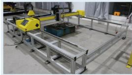
• The fix of the base is heavy Usteel; the cross beam update 80X100MM square steel from the 40X40MM Aluminum, Max support 150KG up.
